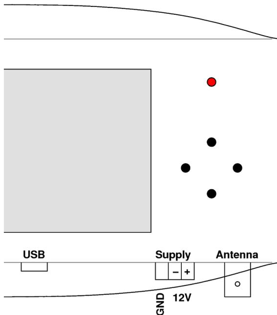
The antenna socket (BNC) can be connected with an active antenna (12V) or a passive antenna (e.g., isolated backstay with passiv-balun).
