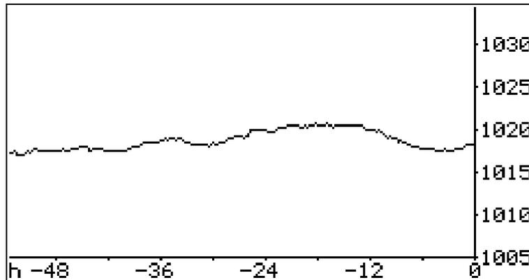
The air pressure of the last 48 hours will be displayed. The actual air pressure is located on the right of the diagram.
