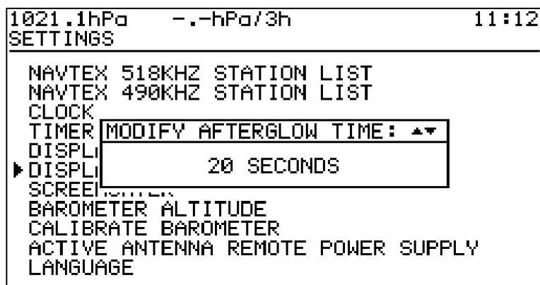
The afterglow time determines, how long the backlighting remains enabled after the last keystroke. The adjustment range is between 0 and 60 seconds.
